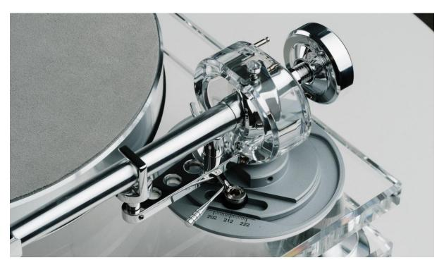
The M6xTT's new 9" tonearm is an ultra-low resonance design with a conical aluminium tonearm tube and a transparent acrylic bearing ring. The arm is fully adjustable for azimuth and VTA settings, and comes equipped with two TPE-damped counterweights to support a wide range of cartridges. The tonearm is connected to a phono stage by a standard 5P DIN cable, allowing for easy cable upgrades in the future.
