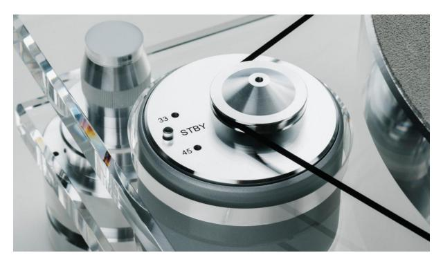
The drive motor allows for push-button changes between 33 and 45rpm speeds, and houses within its structure a sophisticated DC-driven AC generator. This construction means that the frequency and voltage feed for the motor are generated from scratch within the motor assembly, rather than being reliant on the external power supply.
